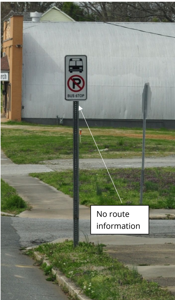
FIGURE 22: SALISBURY TRANSIT STANDARD BUS STOP SIGN
